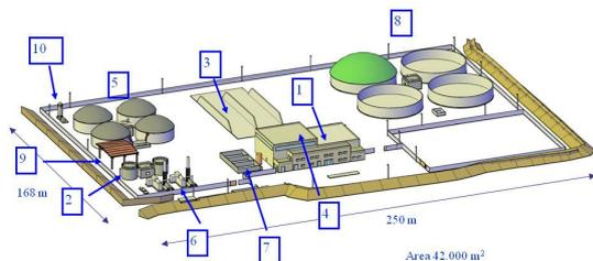
**Figure 5.** Castellone plant layout: (1) reception; (2) manure storage; (3) agricultural substrates storage, (4) pretreatment and sanitation; (5) anaerobic digestion; (6) cogeneration (7) biofilter; (8) digestate storage; (9) rejects storage; (10) biogas flare
